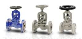
GV-16K GV-25Z GV-40K Body GG-25 Cast Iron EN-GJS-400-18LT (5.3103) 1.0619 Connection Flanged Flanged Flanged Max. Work. Temperature 250°C 250°C 350°C Max. Work. Pressure 16 bar 25 bar 40 bar
