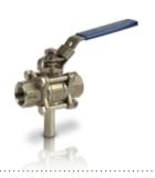
**Body Material** Ball Material Body Gasket Ball Seat Connection Type Nominal Pressure (PN) Max. Operating Temp. Stainless Steel AISI 304 Stainless Steel AISI 304 PTFF R-PTFE (15%) Threaded and Flanged 40 bar -50/+210 °C
