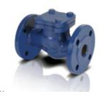
Body Material GG-25 Cast Iron GG-25 Cast Iron Cover Disc Material Spring Material Stainless Steel AISI 304 Stainless Steel AISI 304 Gasket CrNi laminated pure graphite Connection Type Flanged Nominal Pressure (PN) 9,6 bar Max. Operating Temperature 100°C 300°C
