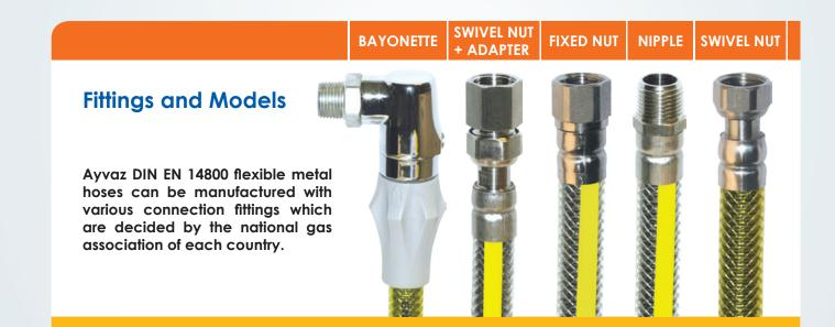
Swivel Nuts: Nut in AISI 304 (1.4301) as per ISO 228 G 1/2 threadInternal Parts: Internal parts in AISI 304 (1.4301)Nipple: Nipple in AISI 304 (1.4301) stainless steel as per ISO 7/1 R1/2 thread
