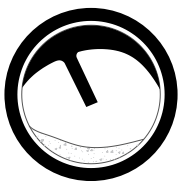
Figure D/Steam Leak The passing steam has significantly suppressed the water surface. Steam filled the area between the deflector and the water surface. That means, the steam trap is leaking steam.
