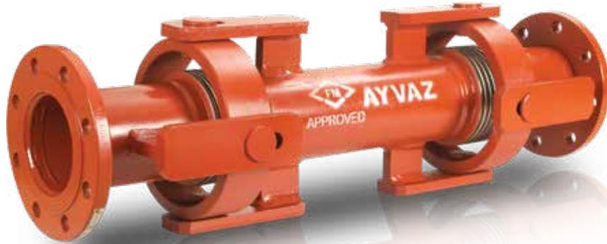
Gimbal type expansion joints are designed to permit angular rotation in any plane by the use of two pairs of hinges affixed to a common floating gibal ring.
